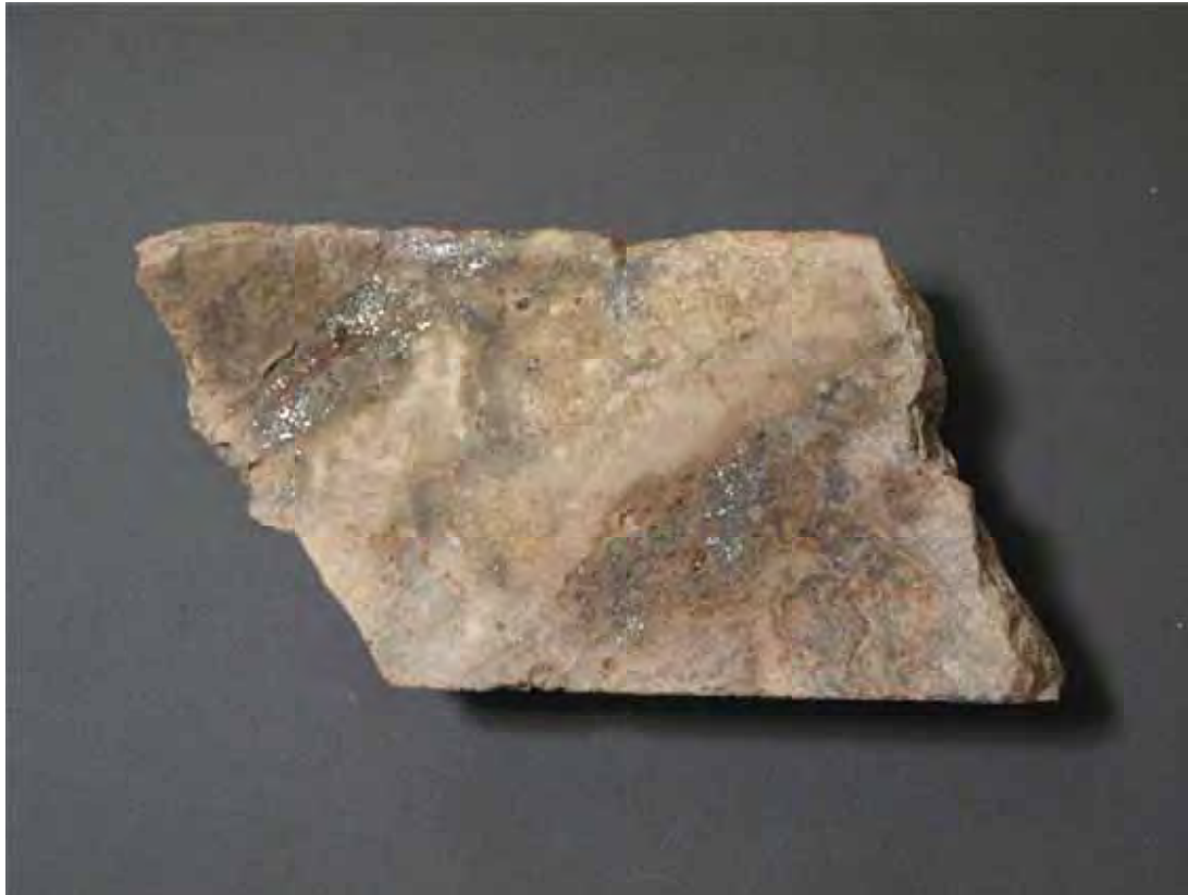
Figure 9-7: Photo of Portion of High Grade Vein in Core from Drillhole 09COM043
