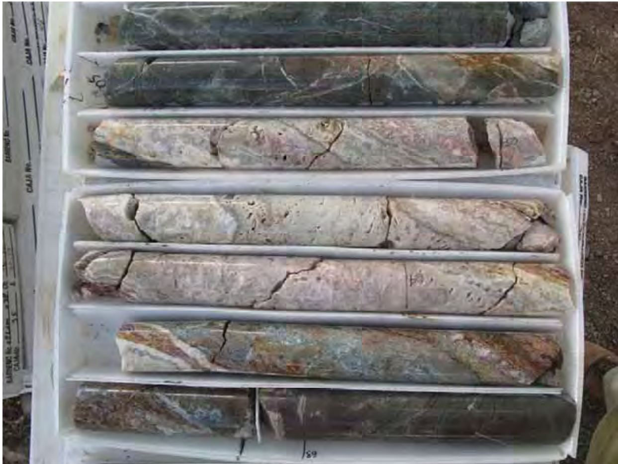
Figure 9-10: Photo of one of the veins cut by drill hole 09COM048 at El Orito. Silver sulfides visible as dark patches just right of 64 meter mark (HQ diameter core).
